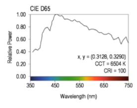
Artificial daylight fluorescent tubes and fittings are available from specialist manufacturers. *This information comes from JUST Normlicht of Germany*. (Other manufacturers, Osram, Philips etc. also produce 6500K tubes, but the x y coordinates may differ from the standard.)
