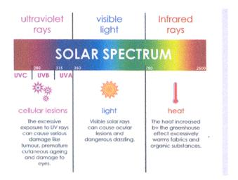
**UVC Radiation** has a wavelength between 200 nm and 280 nm. It is short wave radiation, rich in energy, absorbed by the ozone layer in the atmosphere.
